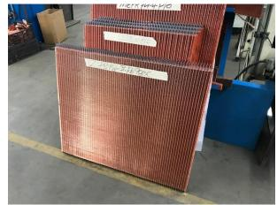
Header Installation: Headers are installed onto cores completing the core assembly.
