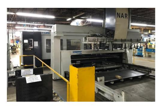
Fabrication Capability: LVD 2K Watt Laser Work Center, LVD CNC 3-Axis Press Brakes.
